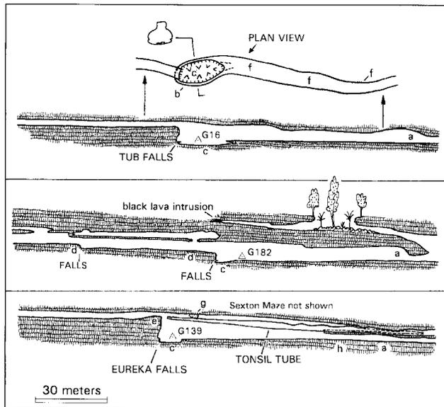
**Figure 15. Some projected profile views of typical lava falls. Sexton portion. (a) beginning area of backcutting, (b) secondary passage width enlargement, (c) plunge pool, (d) the development of a stepped floor with any significant slopes taken up by falls, (e) lip build-up, (f) primary widening, (g) a connection between the main passage and the embryonic Sexton maze, (h) a stacked passage below a fall.**
